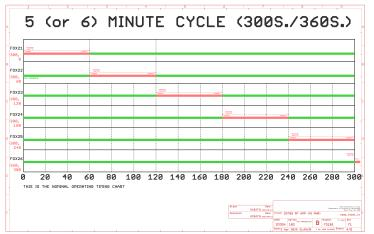
RED bar indicates transmitter active GREEN bar indicates transmitter idle
