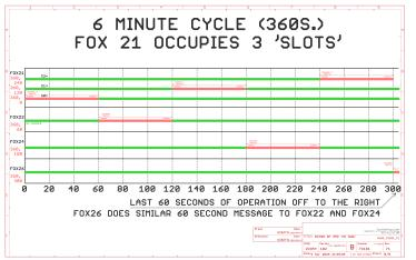
Some of this shows up on 144.250MHz 5 transmitters on 6 minute period, one does double duty
